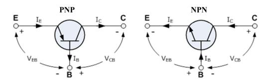
The symbols for both the NPN and PNP bipolar transistor are shown above along with the direction of conventional current flow. The direction of the arrow in the symbol shows current flow between the base and emitter terminal, pointing from the positive P-type region to the negative N-type region, exactly the same as for the standard diode symbol. For normal operation, the emitter-base junction is forward-biased and the collector-base junction is reverse-biased.
